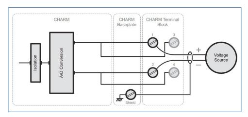
Simplified Circuit and Connection Diagram for LS AI 0-10V DC Isolated CHARM.
