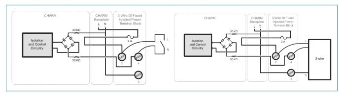
Simplified Circuit and Connection Diagrams for LS DI 120V AC Isolated CHARM with 3-wire DI Fused Injected Power Terminal Block.
