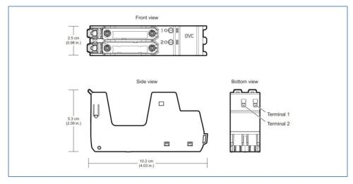
LS CHARM Redundant DVC Terminal Block.
