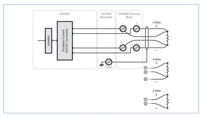
Simplified Circuit and Connection Diagrams for LS RTD CHARM.
