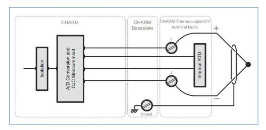
Simplified Circuit and Connection Diagram for LS Thermocouple/mV CHARM with Thermocouple/mV Terminal Block.
