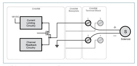
Simplified Circuit and Connection Diagram for LS DO 24V DC ETA CHARM.
