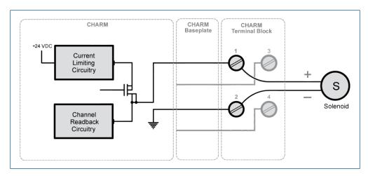
Simplified Circuit and Connection Diagram for LS DO 24V DC DTA CHARM.
