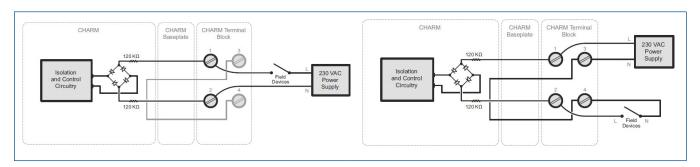
Simplified Circuit and Connection Diagrams for LS DI 230V AC Isolated CHARM.
