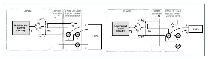
Simplified Circuit and Connection Diagrams for LS DI 120V AC Isolated Plus CHARM with 3-wire DI Fused-Injected-Power Terminal Block.
