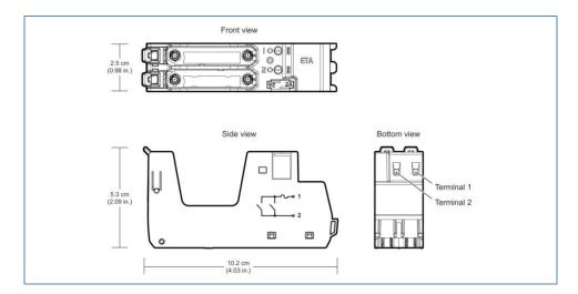
LS CHARM Redundant ETA Relay Terminal Block.
