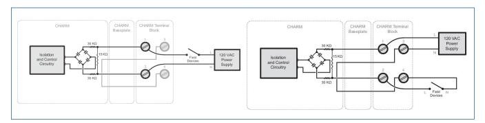
Simplified Circuit and Connection Diagrams for LS DI 120V AC Isolated Plus CHARM.
