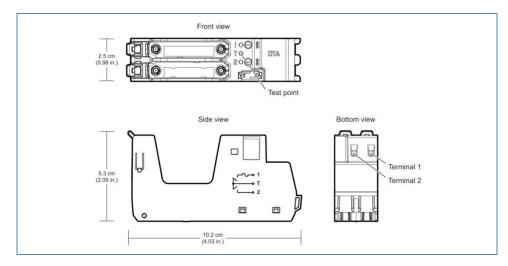
LS CHARM Redundant DTA Relay Terminal Block.
