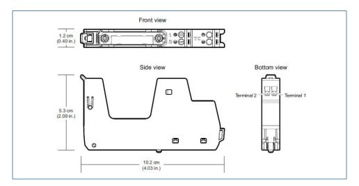
CHARM Thermocouple / mV Terminal Block.
