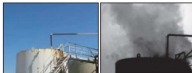
Vented Gas from Oil Storage Tank Visible through Infrared Camera
